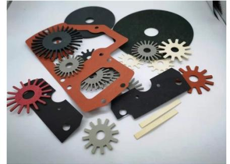
between .0078 " and .375 " thick. It is produced in several grades and colors. The electrical grade of vulcanized fiber is referred to as fish paper. Vulcanized fiber has superior flatness, high mechanical strength, and excellent resistance to heat and cold. It is light weight, has excellent tear resistance, and can be machined with standard tools. It can be machined, punched, slit, threaded, formed, molded and wound into tubes for literally countless applications.
